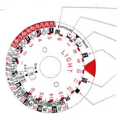
"U" and "O" positions permit exposure determination by measurement of darkest and brightest objects.
